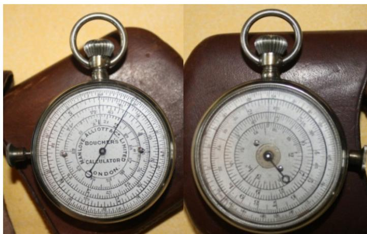
*Figure 31: A second example of Manlove Alliott & Co Limited Boucher Calculator*
