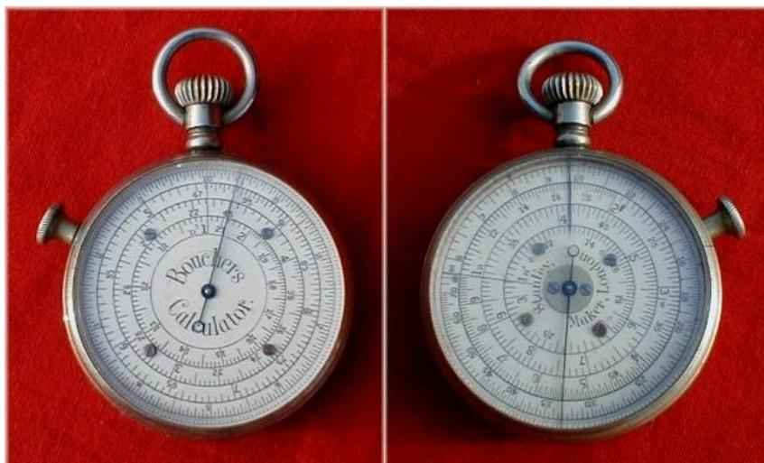
Figure 34: Boucher calculator made by W.F. Stanley
