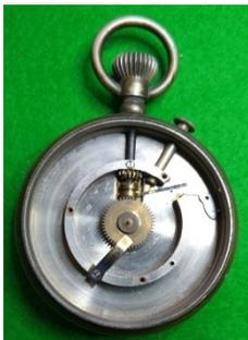
Type 15 is typical of most 'fat' Calculigraphe in that there are three screws to each front and back, however these are noticeably larger than the standard tiny screws that feature on most other models.
