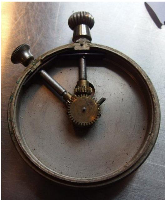
Figure 12a: Internal view of the different very early Boucher calculator
